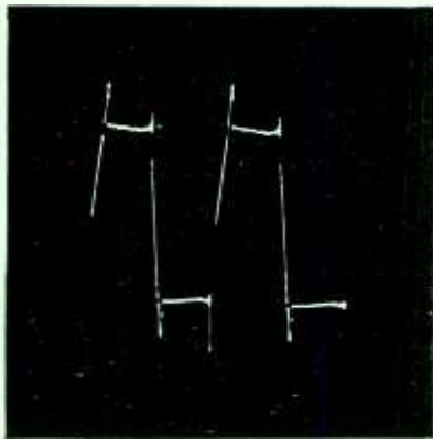
Fig. 2—VIBRATOR OSCILLOGRAM— Waveform of a good auto vibrator. Flat-topped curve indicates positive contact of points. Magnitude of sharp corner peaks are tell-tales of degree of sparking at moment of contact
